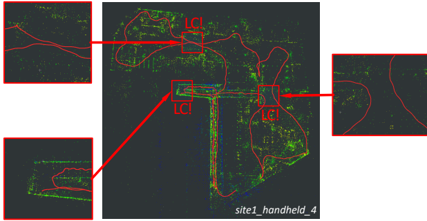
Fig. 4: Multiple detected closed loops from site1_handheld_4 sequence in Hilti SLAM Challenge 2023. Accumulated drifts are significantly reduced, ensuring enhanced accuracy and robustness.
