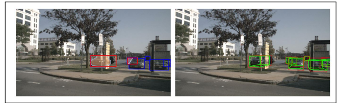
Fig. 7. If the annotators label the occluded 2D parts, our model will also consider occlusion during the refinement.
