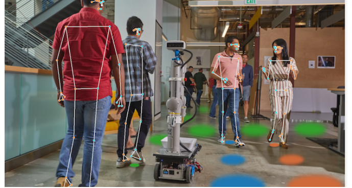
Fig. 1: A service robot navigating a busy office space. To do so it anticipates human motion using human-position and visual features such as head orientation or 3D skeletal keypoints.
