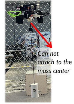
(a) External force model (b) Mount point mismatch
