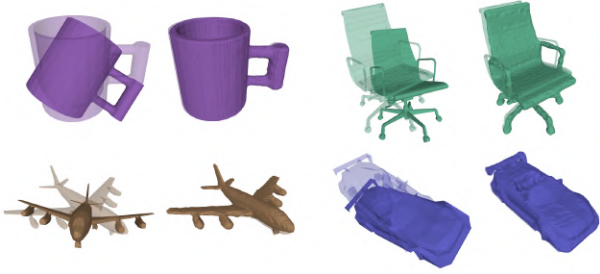
Fig. 3. Example shape alignment results. The meshes on their canonical poses are shaded. Reconstructed meshes are on the right, given perturbed meshes are on the left. Post-training, shapes are aligned very closely to their canonical poses.
