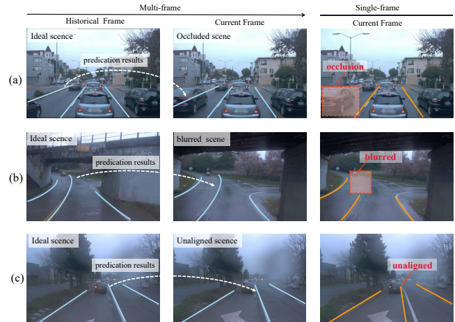
Fig. 1. Motivation behind Bi 2 Lane: the predictions from the historical frame serve as anchors in the current frame, enhancing single-frame resilience to environmental variations. For example, (a) illustrates the supplementation of an occluded lane from the historical frame. (b) illustrates the process of patching the blurred lane from the historical frame. (c) illustrates the lane alignment achieved through acquiring historical lane information.
