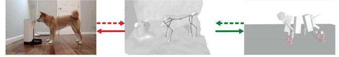
Fig. 3. Physics-informed 3D reconstruction pipeline: Differentiable rendering from a monocular video (left) and differentiable physics simulation (right) update key-point motion estimates (middle). Solid red and green arrows represent rendering and physics-roll-out costs; dashed arrows are corresponding gradients.
