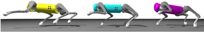
Fig. 6. Comparison between the reconstructed key-point reference (yellow), optimized reference (teal, ours), and learned imitation policy [4] (purple).
