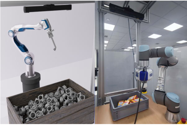
Fig. 6. Comparative experimental setups showcasing robotic grasping. On the left, a model-based grasping scenario is depicted, utilizing a Diana7 robot and a Photoneo L camera for industrial part manipulation. On the right, a half-model based grasping approach is illustrated, employing a UR5e robot and a Photoneo M camera.
