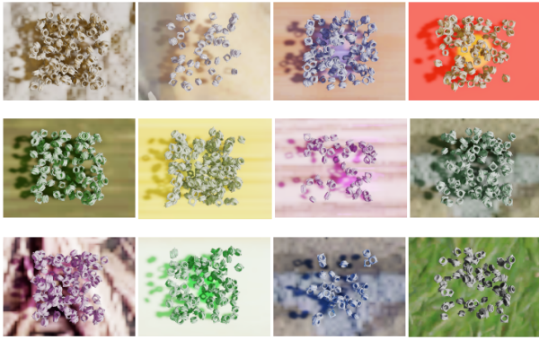
Fig. 5. The creation of a domain-randomized dataset using the Isaac Sim platform. The dataset generation features varied scene backgrounds, object numbers and poses, and lighting conditions in terms of intensity and color. Each parameter is randomized to increase the diversity of the dataset.
