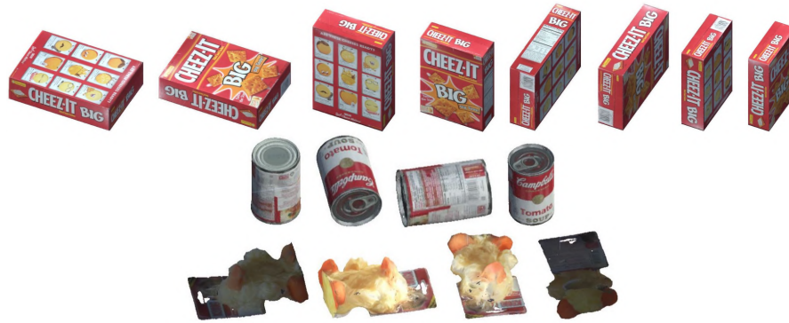
Fig. 2. An illustrative example of the orientation configurations for three objects with different geometry and texture properties to assess the performance of the vision pipeline in phase 1 of stage 1. Cheeze-it Cracker box (first row) has more configurations with respect to the other two due to its symmetry along all the three principal axes ( x,y,z ) and its diversified texture; Tomato Soup can (second row) has just four configurations due to its cylindrical symmetry; and Kong duck dog toy (last row) can only be placed laying on the floor of the box since it has only two different stable poses on a table but presents different visual appearance depending on the side it is lying on.
