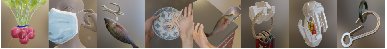
Fig. 1: Soft fixture scenarios: (1) radishes held together with a rubber band, (2) putting on a mask, (3) hooking a frozen fish with a fishing hook, (4) catching a starfish with a bowl, (5) scooping a fish with a shovel, (6) grasping a chain of transfusion bags, (7) manipulating a Rubik cube with two grippers, (8) snap lock mechanisms. The examples include textures and meshes by [6]–[23].
