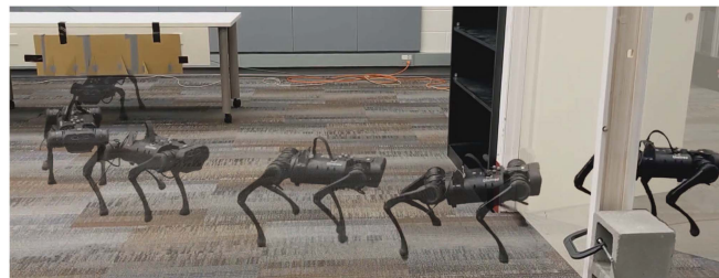
Fig. 1. Our framework allows robots to learn complex environment interactions with a recursive hierarchy. The image shows a motion frame of the robot crawling under a table, reaching the door, pushing it open, and walking through it to reach a target location.
