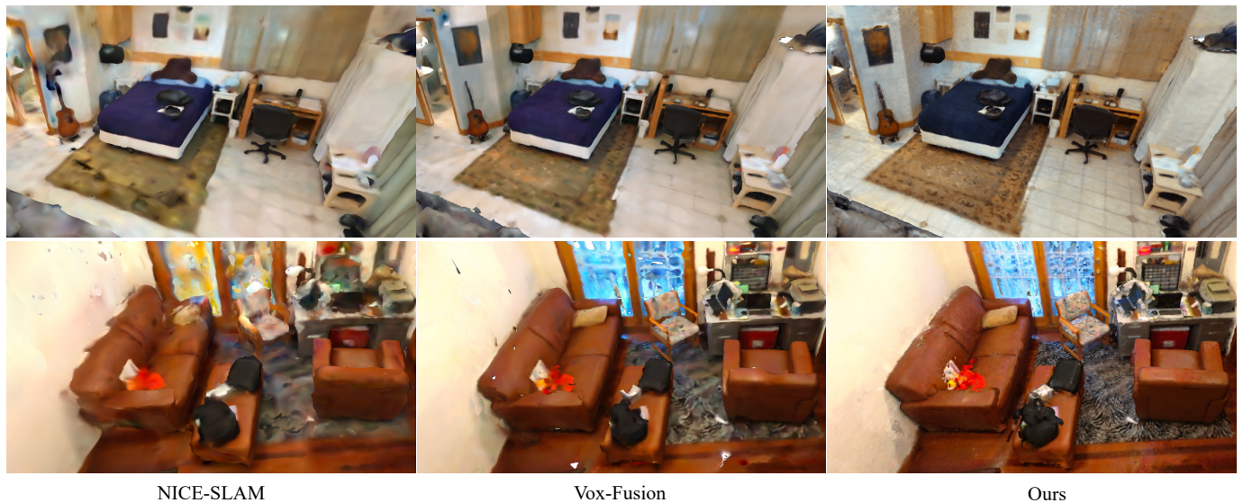
Fig. 8. Textured mesh on the ScanNet dataset [22]. Our method produces more accurate geometry and higher-fidelity textures.
