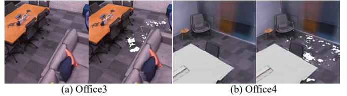
Fig. 11. Ablation study on expanded voxels allocation technique. (a) and (b) show results about Office3 and Office4 of Replica [21], respectively. This technique can produce fewer holes during the mapping (Use: left; No use: right).
