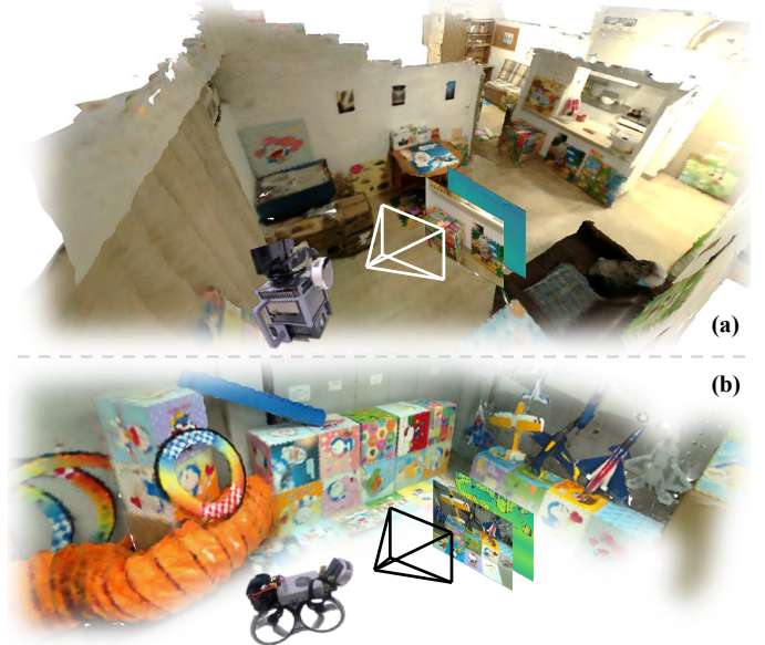
Fig. 1. We tested our methods on a handheld device (a) and quadrotors (b). Our method builds a high-quality map in real-time on edge computers and can support robotic applications.
