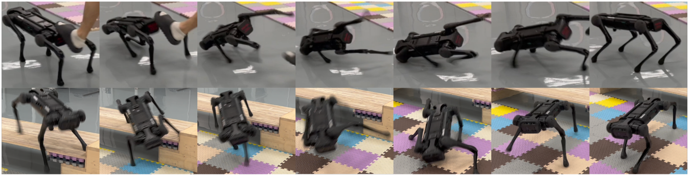
Fig. 4: Snapshots of the robot’s recovery when it missed a step or got pushed. The robust policy learned through risk-sensitive RL makes the robot retain balance rapidly when encountering intense disturbance.
