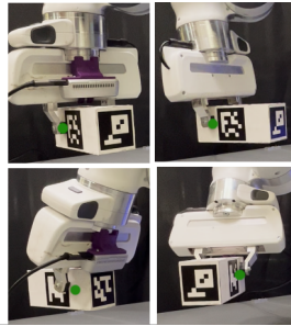
Fig. 10: Robot Demo [Left] Grasp success rate for two novel blocks. The baseline method (@0) only uses visual information while the GNP method (@10) uses 10 adaptation interactions. COM is relative to the object center. [Right] After 10 adaptation grasps, the robot consistently grasps the object near the CoM (green dot).
