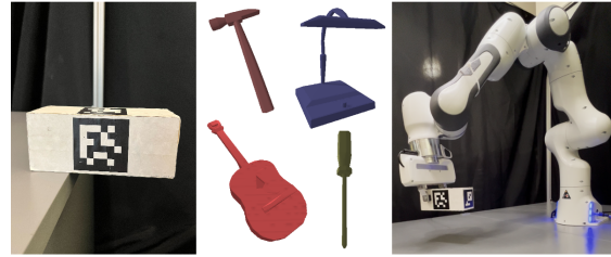
Fig. 1: Our method allows a Panda (right) to infer unobserved properties of objects based on interaction history. This allows the robot to efficiently grasp objects with non-uniform mass distributions such as weighted blocks (left) or ShapeNet objects (center).
