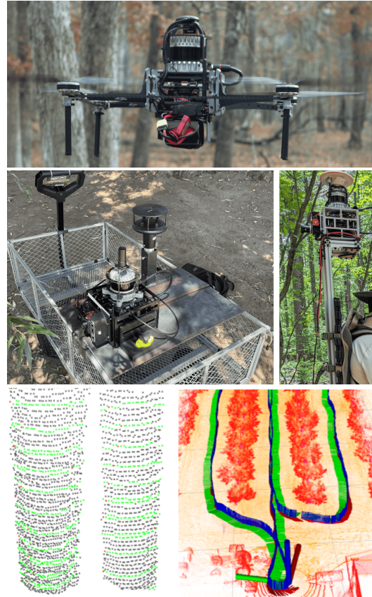
Fig. 1: Overview of the methods for TreeScope data collection. Top: Falcon 4 UAV [6] flying in under-canopy dense forests. Middle: Our sensor platform mounted onto a small cart and human-carried backpack. Bottom left: Forestry tree instance segmentation for diameter estimation. Bottom right: UAV flight in a pistachio orchard. TreeScope is the first semantically segmented LiDAR dataset collected with robotic systems in agricultural environments.
