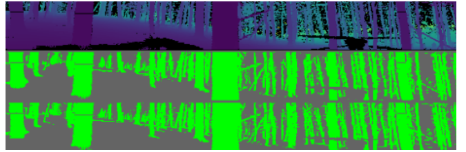
Fig. 4: Segmentation results from the RangeNet++ [15] model. The inference mask (bottom) is compared on a pixel-by-pixel basis to the ground-truth mask (middle) across the test set to compute the segmentation performance metrics. Top : Range image 2D projection of input LiDAR scan. Middle : Ground-truth semantic labels (green pixels are tree stems). Bottom : Segmentation inference from the model.
