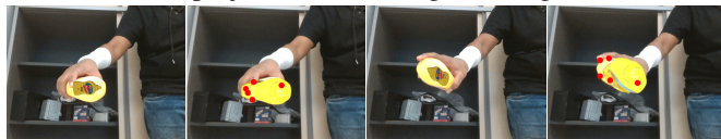
(a) Semi [5] (b) Filtering (c) Semi [5] (d) Filtering Fig. 6: Filtering results. We show that the filtering pipeline can estimate the object pose with just fingertips (red points) as input. It can give robust and continuous estimation even when the purely learning-based method (a, c) fails.
