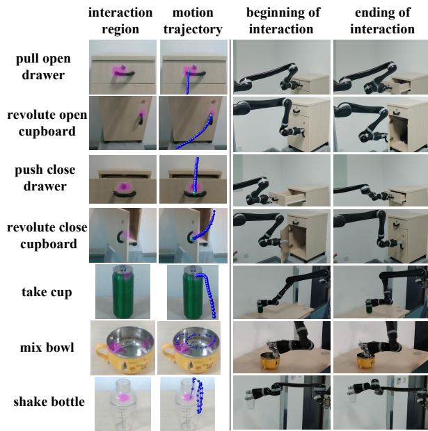
Fig. 8: Interaction with objects in real environments, IRMT-Net predicts the interaction region and motion trajectory to support the interaction of robots.
