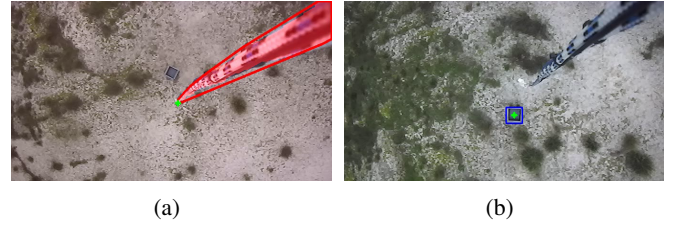
Fig. 3: (a) Detection of the cable. The red-shaded transparent area, surrounded by a convex hull, denotes the detection mask overlaid on top of the original image. The green cross corresponds to the pixels of the load. (b) Detection of the target. The green cross corresponds to the center of the bounding box.
