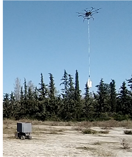
Fig. 1: The multirotor with the cable-suspended load and the UGV deployed in the field.
