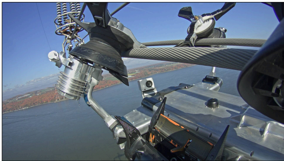
Figure 1. LineRanger rolling on live large river crossing spans.
