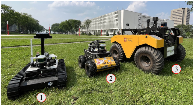
Fig. 4. Three different commercial platforms that were used for the experimental work: a Superdroid HD2 (1), a Clearpath Robotics Husky (2), and a Clearpath Robotics Warthog mounted on wheels (3). The platforms weigh 80 kg, 75 kg and 470 kg, respectively.
