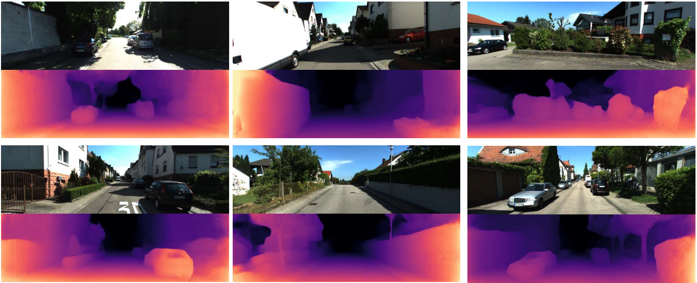
Fig. 3: Prediction result sample from KITTI-360 dataset. Pixels colored in white are expected to be closer to the camera. The pictures demonstrates the network’s ability to distinguish close-up objects against backgrounds.
