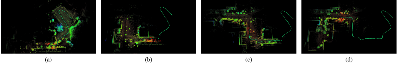
Fig. 4. Subfigures (a) to (d) show smooth transition and the localization path passing through 4 consecutive block maps on nclt.2 . Our switching strategy is able to maintain spatial continuity with good performance.
