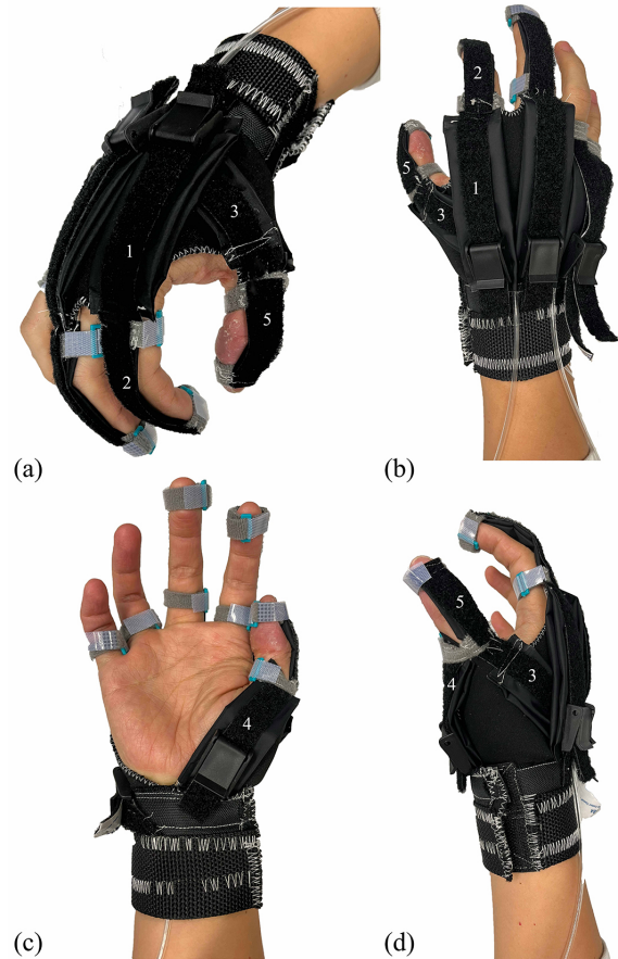
Fig. 1. The overall design of the extension glove is depicted in the figure. The serial numbers, 1, 2, 3, etc., correspond to the straps that will be consistently referred to throughout the entire paper. (a) Perspective view: The glove features an adjustable belt system that can accommodate users with different hand sizes. Its one-sided wearing design allows for convenient and quick application and removal, particularly beneficial for spastic hands. (b) Back of hand side view: Each MCP joint is connected to strap 1 and X-pouches for extension, whereas the PIP and DIP joints share strap 2 and a corresponding X-pouch for extension. (c) Palm side view: Strap 4 and an X-pouch are positioned on the thenar to facilitate abduction of the CMC joint. (d) Thumb side view: Strap 5 and an X-pouch are utilized to extend the IP joint, while the MCP and CMC joints share strap 3 and an X-pouch for extension.
