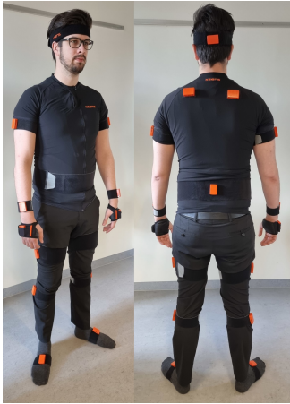
Fig. 2. Xsens tracking suit with IMUs
