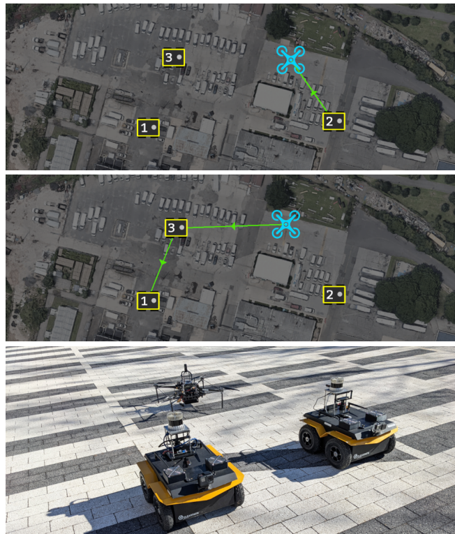
Fig. 1. Top: Visualization of the real-world experiments using MOCHA to enable communications between a UAV and three UGVs. The UAV first communicates with robot 2 and exchanges information. Middle: The UAV acts as a data mule transmitting robot 2’s information to robot 3, which itself propagates the information to robot 1. Bottom: Autonomous robots during our heterogeneous exploration experiments: the Falcon 4 UAV and Clearpath Jackals.
