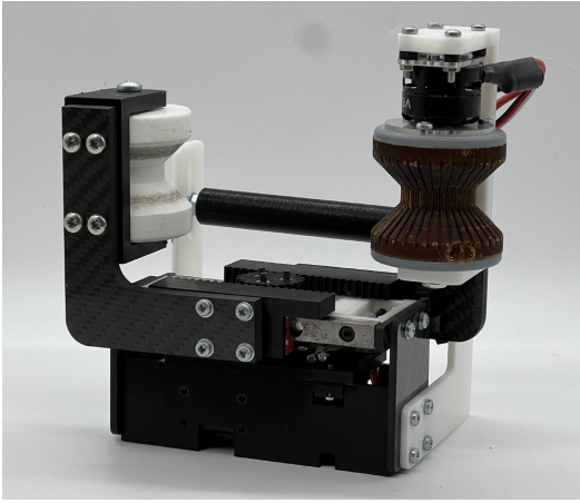
Fig. 3: Prototype of the active rolling gripper module used for perching.
