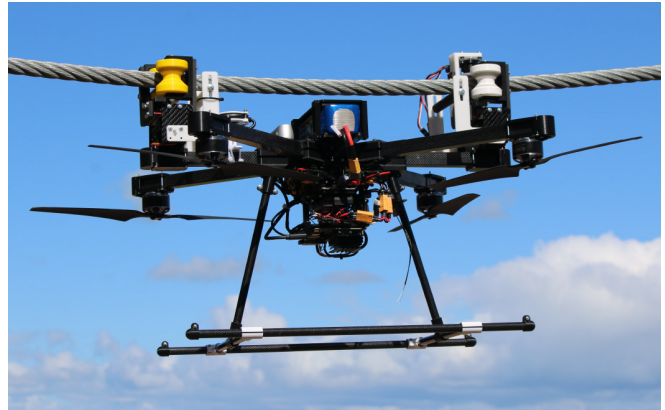
Fig. 1: The proposed perching and rolling capable UAV attached to a power line through its ratcheting, serial elastic parallel jaw grippers.
