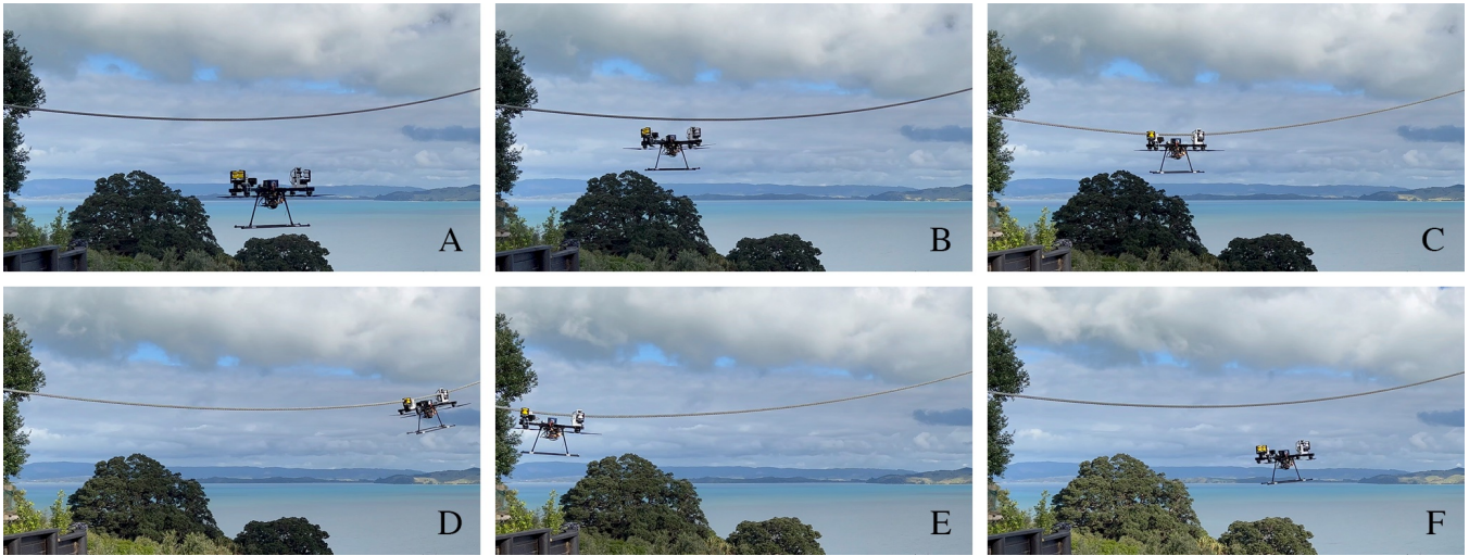
Fig. 6: Instances of the autonomous perching and unperching experiments that have been conducted with the proposed grasping and perching capable powerline inspection UAV platform. The UAV approaches the powerline (A) and begins to track the line (B). It then autonomously perches (C), and is able to remain perched indefinitely. It can then translate along the powerline (D, E) and when applicable, autonomously unperch (F).
