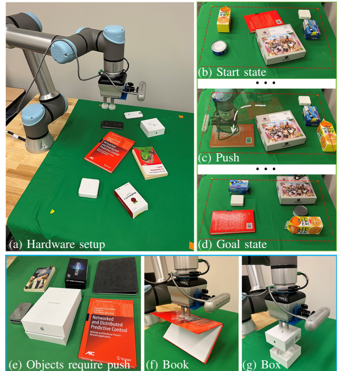
Fig. 1: (a) Overview of system setup, a camera is mounted on the end-effector for perception. (b) - (d) An example case and an intermediate step in solving it. (e) Example objects requiring push . (f) pick-n-place may break the book. (g) pick-n-place will separate a box, failing to pick it up.
