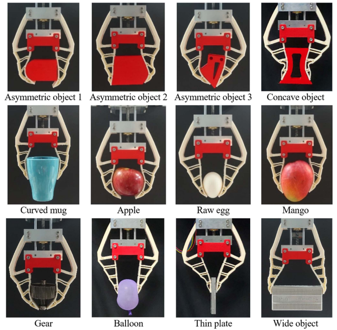
Fig. 11. Test results for grasping a variety of different objects using the highly self-adaptive gripper with the multi-infill density fingers.
