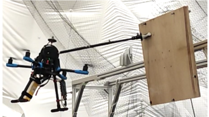
Fig. 1: A quadrotor-based aerial manipulator is pushing on a flat oriented work surface.
