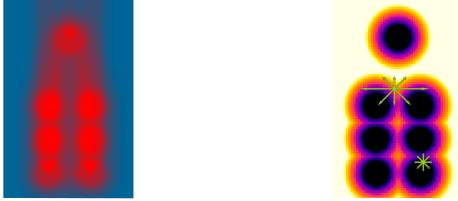
Fig. 3: Assembled safety cost grid ( SC_i ) with k_a = 0.3 , k_b = (v_{sat}(d_{obs})) . Low is in black 0.2, and k_c = 0.5 (arbitrary). and high in yellow. Green Red is 1 and blue is 0. arrows indicate v(d_{obs}, \theta) .
