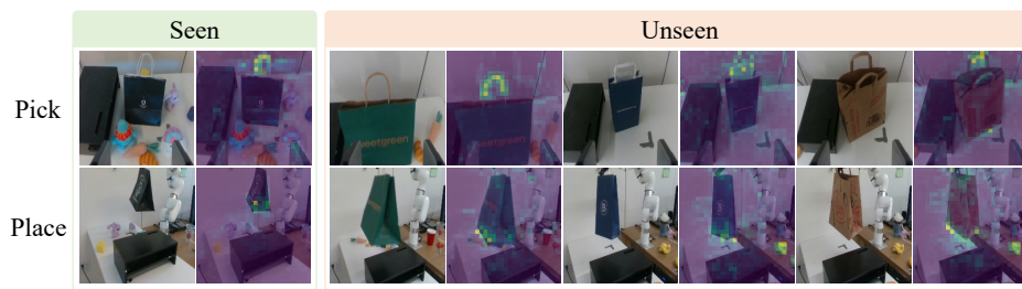
Fig. 6: Visualization of the attention on the pre-trained features by the last adapter during the Place Bag task. The attention focuses on important regions that are consistent across even unseen instances, e.g. the bottom of the bags are highlighted when placing.
