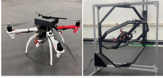
Fig. 2: The drone used in the experiment and the system called FFT-GYRO 450 which restricts the drone to rotational motion
