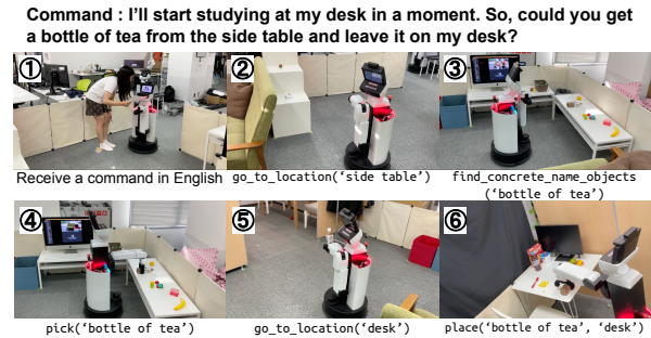
Fig. 1: GPSR task execution example by our system. Commands are converted into a sequence of skills and executed one by one.
