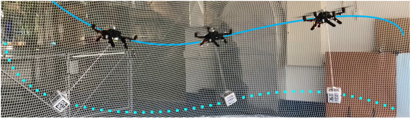
Fig. 1: Intel Aero quadrotor carrying a cube-shaped slung load attached by a string in a dedicated motion capture arena.
