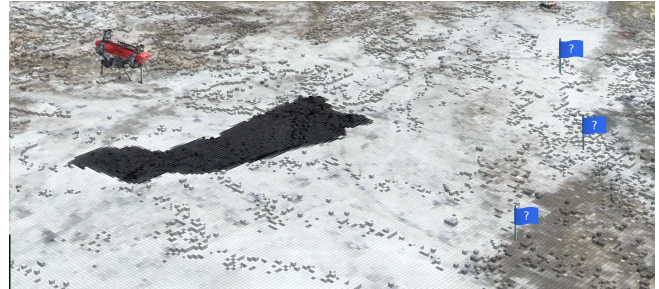
Fig. 1. ANYmal C [7] in the Spanish Tabernas desert during an analog mission. The world is depicted in the VDBMap with additional information. The possible exploration goals are marked with blue flags. The robot needs to prioritize the goals according to the possible information gain.
