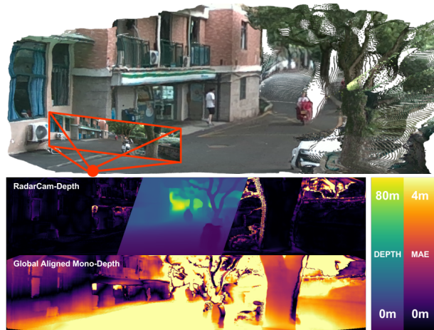
Fig. 1: Top: 3D visualization of the metric depth estimation from our proposed RadarCam-Depth; Middle: Our metric depth estimation overlaid on corresponding error map; Bottom: Error map of Mono-depth after scale-aligned to Radar points. Our depth estimation exhibits exceptional metric accuracy and fine details.
