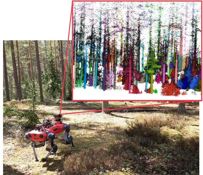
Fig. 1: Instance segmentation results on data collected with a mobile robotics platform in a forest near Evo, Finland. On the left, we show the ANYmal platform, which was used for data collection, and on the right the segmentation results of our approach on the collected data. Different colors of points indicate different instances.
