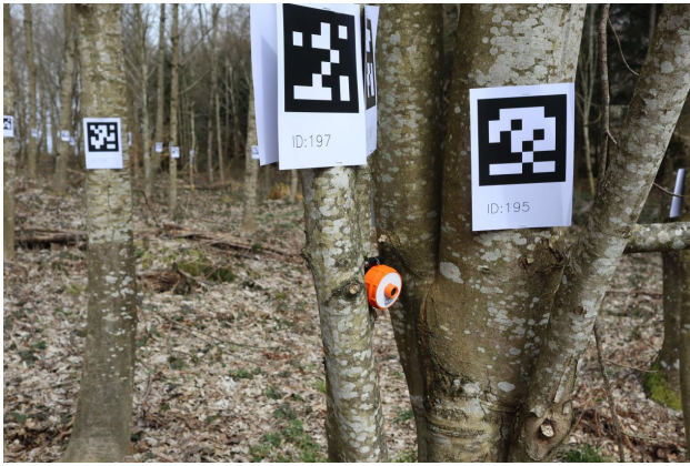
Fig. 3: An image of one of the forest plots in Switzerland. April tags are placed on individual trees to allow easy association of the measured traits.
