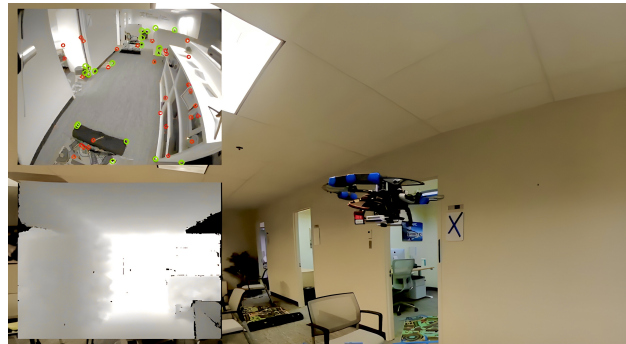
Fig. 1: Our Falcon 250 Platform [8] exploring an office building. Falcon 250 is equipped with an Intel Realsense D435i camera, a VOXL board [13], a Pixhawk 4 Mini flight controller, and an Intel NUC 10 onboard computer. The top left window displays the grayscale image with VIO features overlaid, where green/red circles mark high/low-quality features. The bottom left window displays the raw depth image from the RealSense camera.
