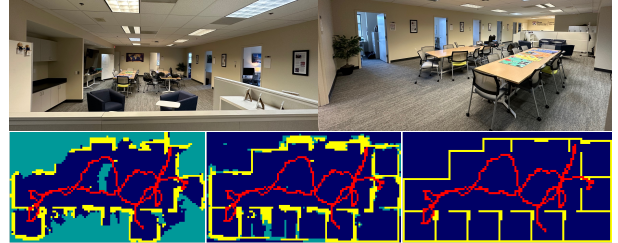
Fig. 8: Representative results of experimentation with the Falcon 250 in an office suite of roughly 10m \times 20m \times 3m dimensions, comprising eight office rooms. On the bottom panel, the right figure shows the ground truth occupancy map that we constructed based on the floor plan. The left figure shows the final observed 2-D occupancy map. The middle figure shows the final predicted map. Free, unknown, and occupied cells are marked as dark blue, light blue, and yellow colors, respectively.
