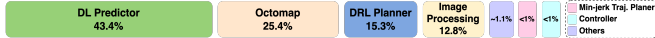
Fig. 7: CPU utilization of the entire software stack. The entire software stack uses 32.7% of the onboard CPU, which is further broken into seven blocks. ‘Others’ includes the utilization of other nodes in ROS.
