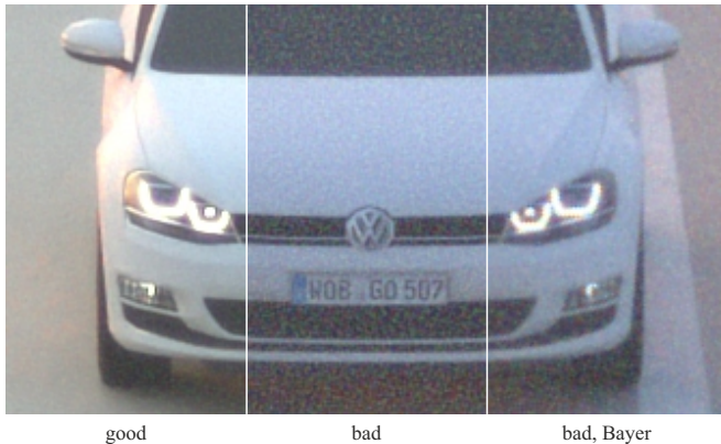
(c) Three of the four qualities (good, Bayer not shown) computed per geometric path tracing result. The “good” quality set has optimal balance and low noise levels. Bad introduces AEC and white balance deviations, lens flares and higher noise levels. Bayer introduces demosaicing effects from a BGGR Bayer pattern (visible, e.g., in the headlight fringes).
