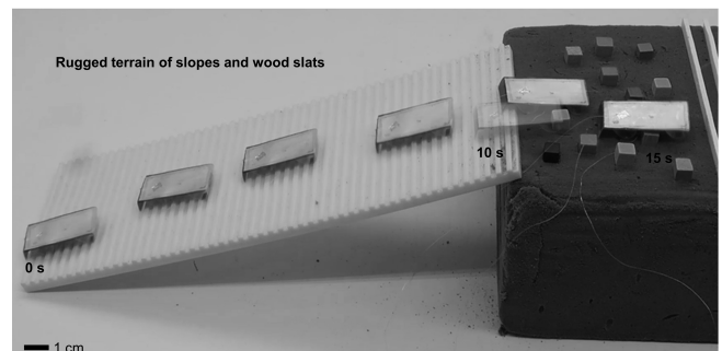
Fig. 8. Multi-locomotion for traversing rugged terrains, including slopes and plummet terrain.
