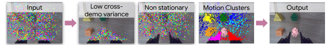
Fig. 3: Active point selection. We exploit the funneling-nature of control to identify relevant points based on their variance, and remove the gripper by filtering static points. Remaining points are used to vote on the motion cluster , which we use to sample 128 points throughout the motion-segment to serve as the salient features for that step of the motion plan.
