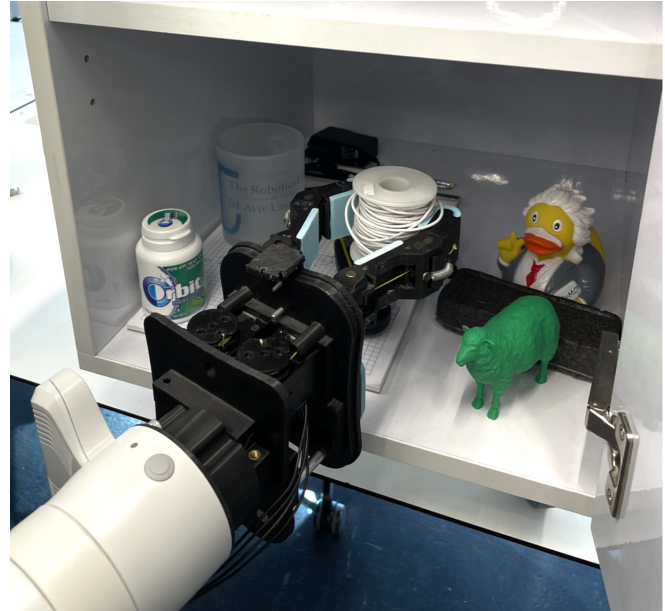
Fig. 1: In-hand recognition of an object in an occluded environment with an underactuated hand where visual perception is not available. The hand relies on kinesthetic perception during in-hand manipulation to either recognize the specific object from a trained set or its general shape.
