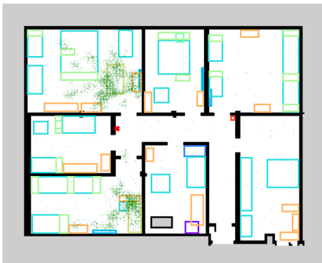
Fig. 5: A failed localization scenario due to ambiguity in both geometric and semantic features. The particles, marked as green dots, are divided between two rooms with similar properties. The weighted-average prediction is marked with a red cross.
