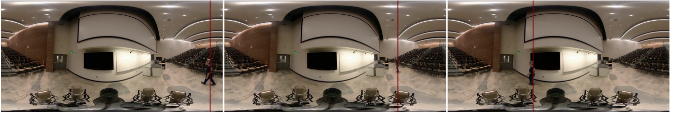
Fig. 2: Frames from the Robot Kidnapper dataset (static robot). The participant wears a hat with ArUco markers [9] used to calculate ground truth radial distance. The RGB frames are used to calculate the ground truth centroid of the person using DeepLabv3+ [10]. Only the audio is used during training. The vertical red lines are the angles predicted by our model in an unseen room. The participant is walking normally in these frames.
