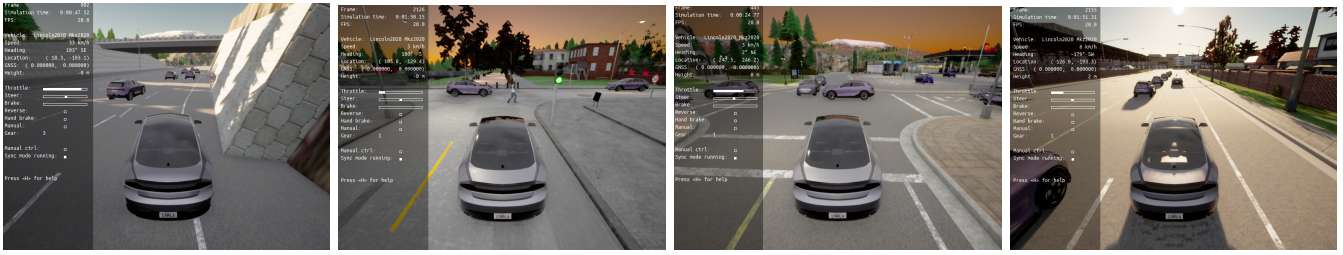
Fig. 4. Testing scenarios (from left): (i) highway merging, (ii) T-junction, (iii) four-way intersection, and (iv) lane changing in dense traffic.
