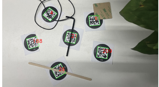
Fig. 1. CopperTag detection example: The CopperTags were occluded by various objects, yet they were all successfully detected
