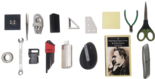
Fig. 8. Parts transported by the gripper. From left to right the parts are: acrylic plate, tweezers, bundled braided cable, PLA triangular prism, 80/20 corner bracket and plate, Post-Its, pliers, scissors, bearing, wrench, Dynamixel, hex keys, bottle of fluid, computer mouse, soft cover book, box cutter. The parts ranged in mass from 17 - 169 grams (from left to right, and top to bottom).
