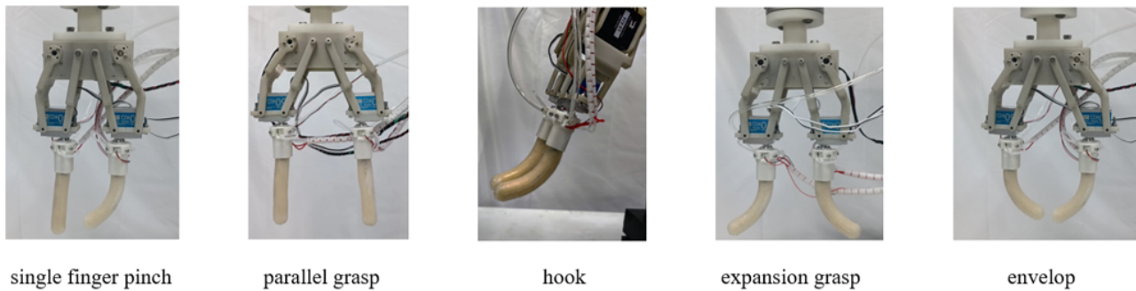
Fig. 6. Multi-modal capture of BSF. The BSF’s multi-mode grasping capabilities are achieved through mode switching, facilitated by the rotation of the root servo and the bending of each finger.
