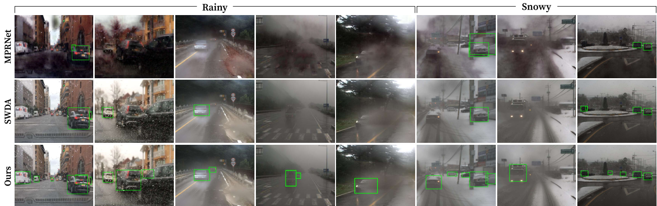
Fig. 3: Qualitative results on real-world target datasets. Compared to other methods, Ours successfully detects the objects even in the presence of severe weather corruption and style variations. Even though MPRNet removes raindrops in the first two images, the detector performance remains low, indicating images generated by the removal network do not consistently help object detection. In the remaining images, the removal network fails to remove corruptions and instead creates some artifacts due to the disparity between real weather data and synthetic weather data, which MPRNet was trained on. While SWDA directly adapts the network to the target domain, it fails to detect objects under severe weather corruption and environmental differences. More qualitative results are available in our multimedia material.
