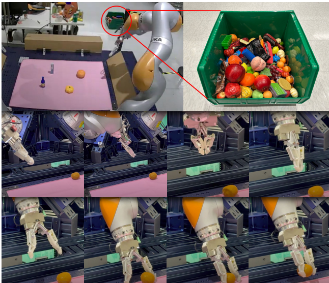
Fig. 5: Upper row : The AB-test setup. Different configurations can vary by the number of objects of the table and their shapes. Lower rows : One of the grasps performed by SARA-ReLU in the low-reachability-area setting (target object close to the robotic arm base), requiring careful PC-input-based control of the robotic arm.
